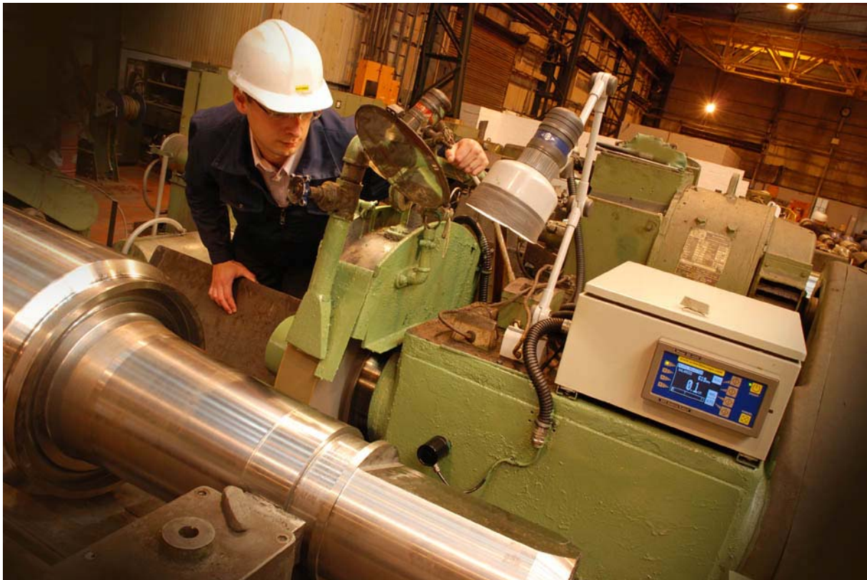
Schmitt Balance System showing the vibration sensor and computer controller installed on a Churchill grinder at Sheffield Forgemasters Engineering Ltd
