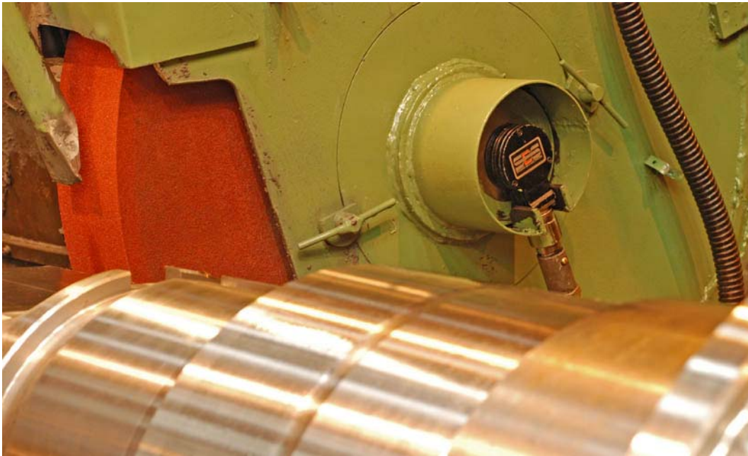
Schmitt Balance Systems balance head installed on a Herkules grinder at Sheffield Forgemasters Engineering Ltd
